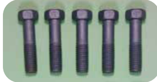
After 2000 hours salt spray test
