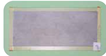
After 2000 hours salt spray test
