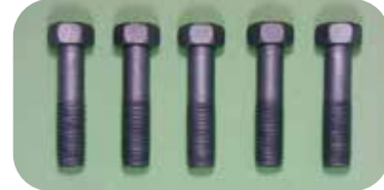
Combined corrosion test (40 cycles)
