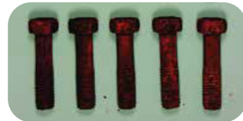
Continued Corrosion Test (15 cycles)
